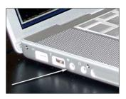
Line in  $\sim$  mini-jack stereo input jack for a stereo microphone
